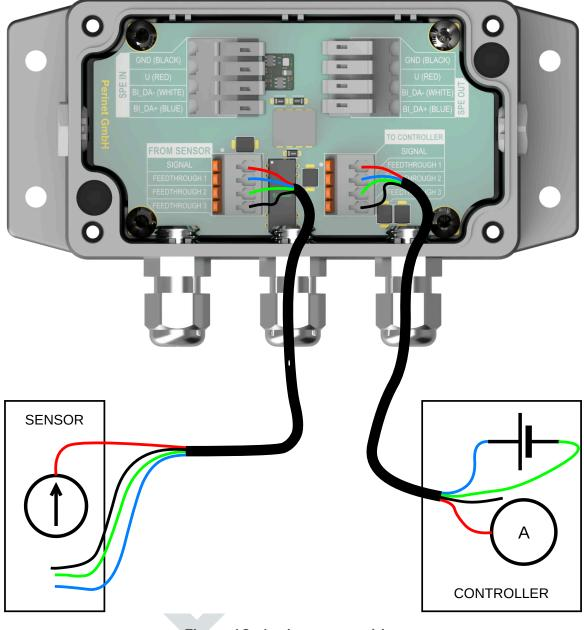
Figure 13: 4-wire sensor wiring
