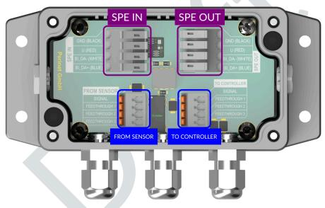
Figure 4: periSNOOP 4-20mA's electrical connectivity.
