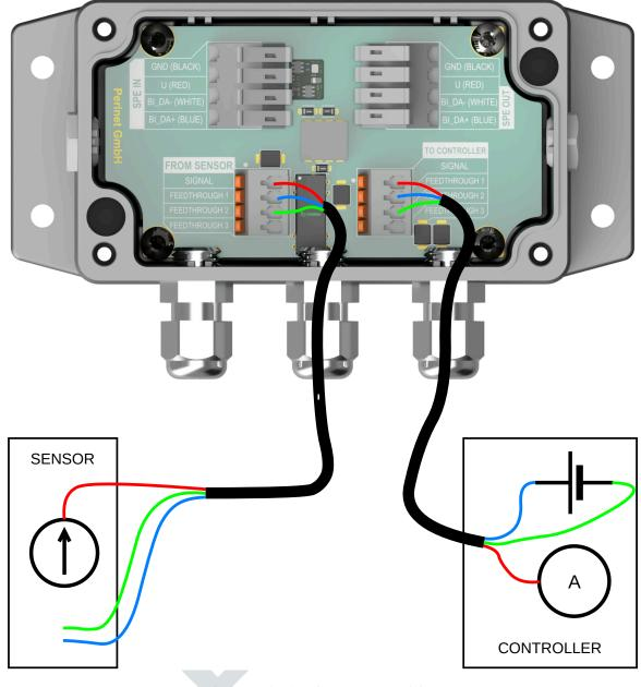
Figure 12: 3-wire sensor wiring
