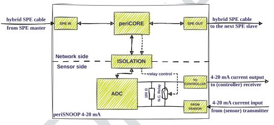
Figure 2: periSNOOP 4-20mA hardware block diagram
