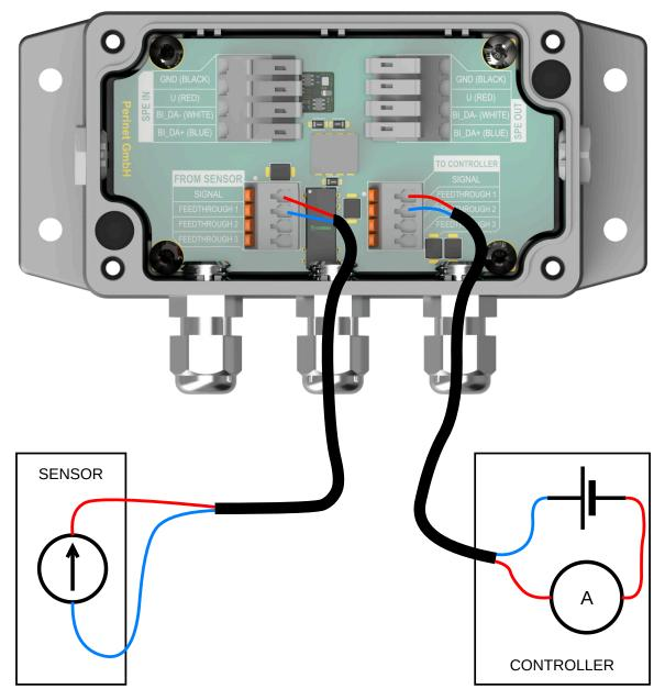
Figure 11: 2-wire sensor wiring
