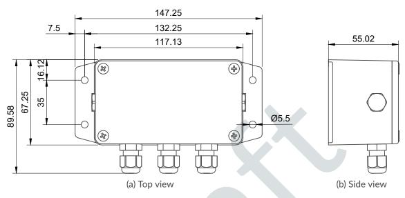
Figure 5: periSNOOP 4-20mA mechanical dimensions drawing.
